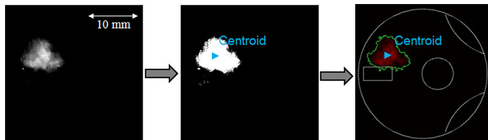
Fig. 4 Processing method for extracting the boundary centroid and locations of flame images
